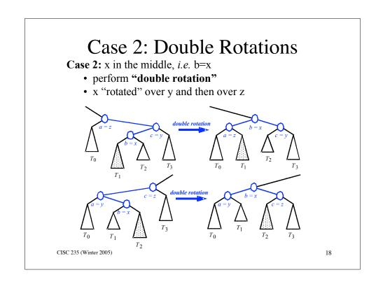
After performing a restructuring after an insertion an AVL is guaranteed to retain BST ordering, and will become balanced.
